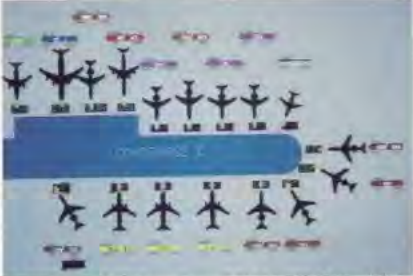
One display available to gate assignment personnel using United's Gate Assignment Display System is an overhead view of one of United's terminals, including a graphic depiction of various types of aircraft at the gates and information about which ones are about to depart.
