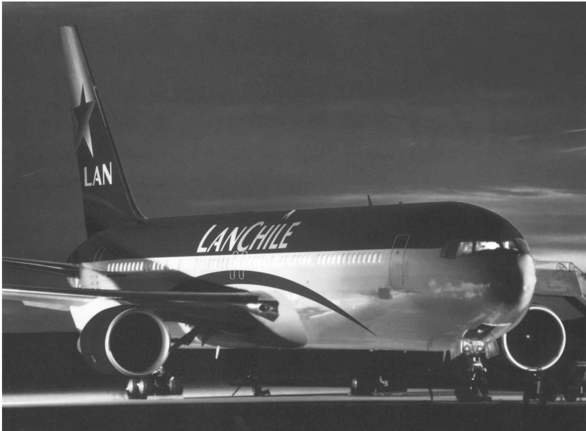
Figure 18-5 Aircraft CC-CZW, a Boeing 767-300ER, Ready for Departure. On the Same Santiago–Miami Flight, This “Combi” Aircraft Can Still Carry 20 Tonnes of Cargo When Carrying a Full 219 Passengers.
