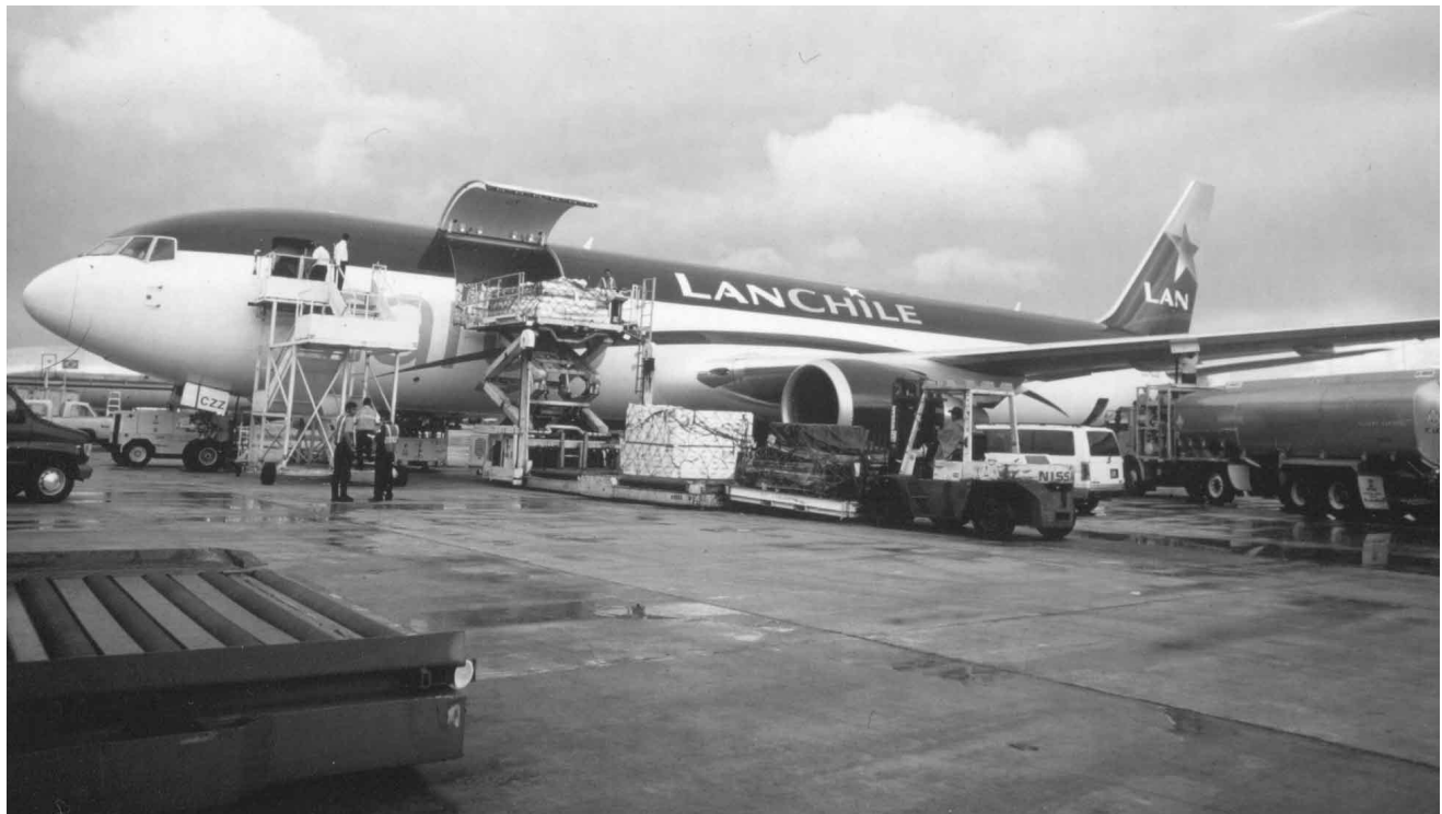
Figure 18-1 Aircraft CC-CZZ, a Boeing 767-300F, Being Loaded with Cargo on the Upper Deck. The Aircraft Can Carry 55 Tonnes of Cargo from Santiago to Miami, an Eight-Hour Flight.
